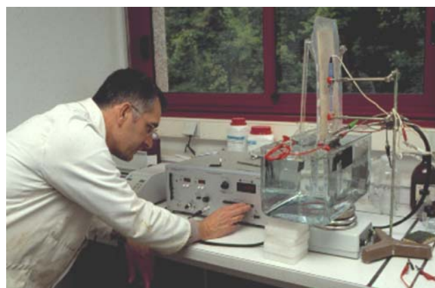
Fig. 12 Consolidative reduction of an altered lead seal still attached to its parchment by cathodic polarisation. The non-immersed parchment is protected in a thermally sealed polyethylene film, while the threads are protected both by a thick layer of CDD and for the outer threads by an extra thermally sealed polyethylene film (credit Arc'Antique)
