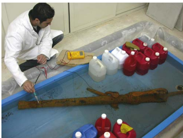
Fig. 6 Monitoring of E_{\text{corr}} vs time on a swivel gun recovered in Maltese waters and stored in 1% w/v NaOH solution. The size of the tank was too big, and containers filled with water were placed in it to limit the volume of the solution to the minimum (credit D. Vella)
